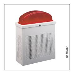
The signalling device SSF/GB is used for external and local alarm signals by intruder alarm systems. The SSF/GB correspond to the VdS guidelines of VdS class C. The acoustic alarm component consists of a tone generator with a power amplifier and loudspeaker. The signalling device SSF/GB also has a strobe light to provide an optical alarm signal.
