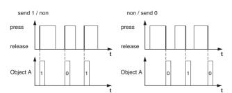
Object A = 1 Byte variable 0-255 value 1 = 255 value 2 = 50 action at pressed/released
