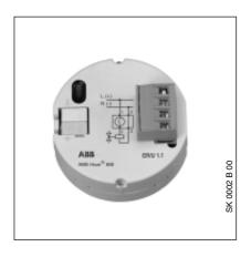
The electronic relay is used to control electrothermal valve drives. It is possible to implement individual room control in connection with the 4-fold universal interface. The device is intended for insertion in a 60 mm, flush-mounted, combined wall and joint box.
