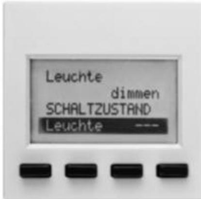
The Info-Display receives telegrams via the *instabus* EIB and allows the representation (LC display) of freely-programmable texts and values.
