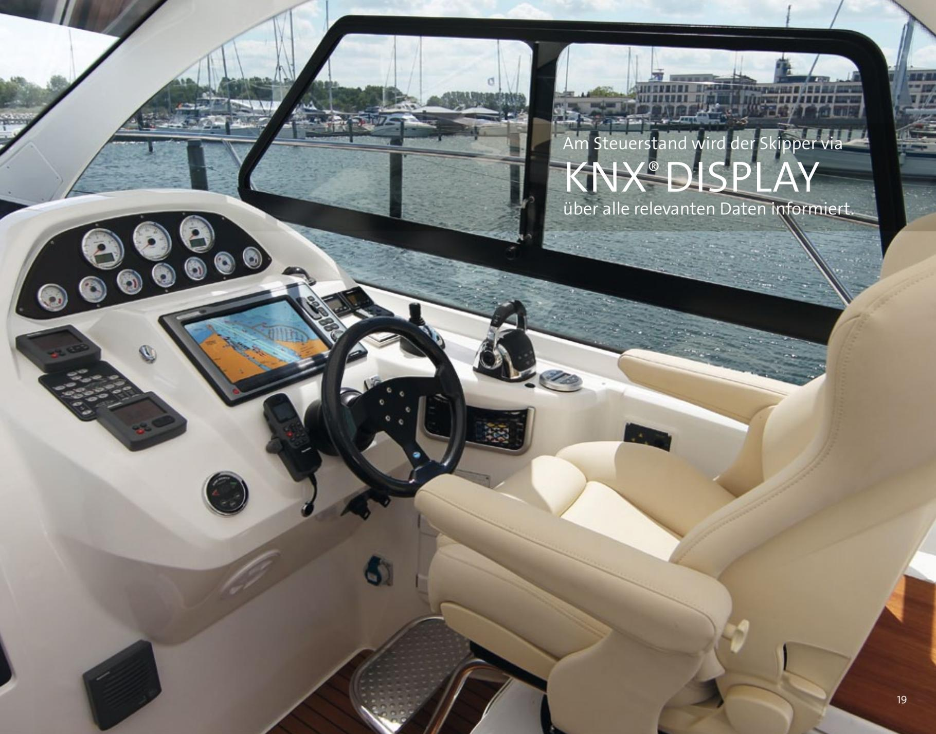
A detailed view of a boat's helm station. The dashboard is white and features a large central display showing a map or chart. To the left of the display are several analog gauges and digital readouts. A black steering wheel is positioned in front of the display. To the right of the wheel is a throttle lever and other controls. The helm station is situated on a boat with a large black frame around the windshield. The background shows a marina with many sailboats and a building on the shore.
